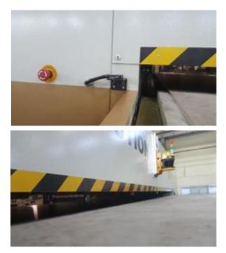
• Full Laser guarding and photo sensors at all trap points ensuring the operators safety
