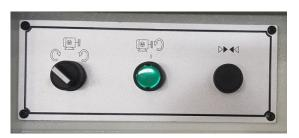
Controls to put the machine on reverse and unjam when excessive cutting pressure is occurred.
